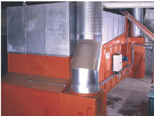
DF 22000 Drier - Specialist industrial application with exhaust dehumidification
