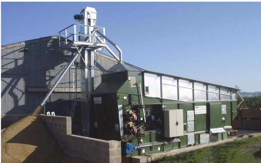
DF 17750 Drier - 19.5 t/yr - typical external installation
