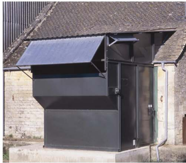
DF 11000 Drier - 12t/hr - typical part external installation, well adapted to old farm building
